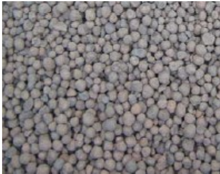
Lytag has eight times greater hydraulic conductivity than gravel
